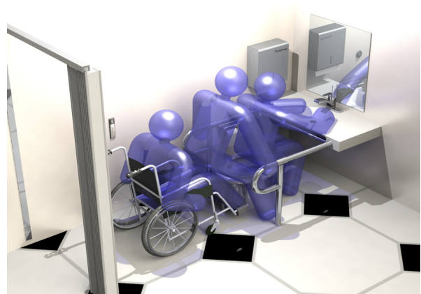
Figure 2. Performing Usability Test Using Front-Entry Sitting Bathroom
