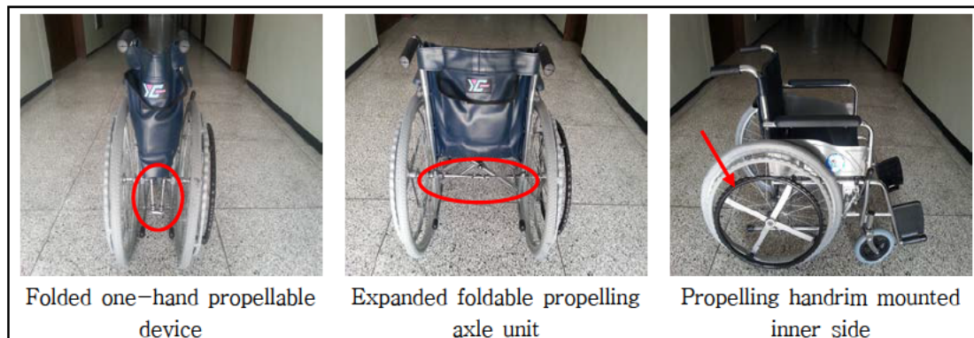
Figure 1. Developed One-hand Propellable Device Mounted on Standard Manual Wheelchair
