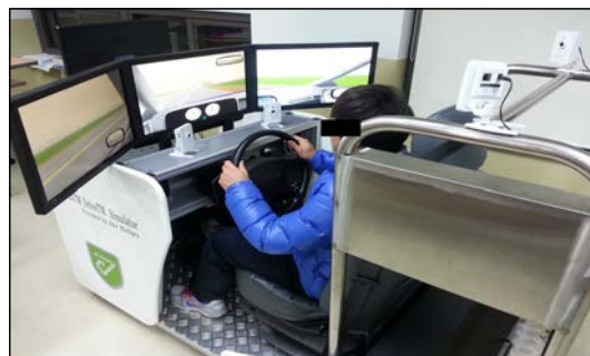
Figure 2. STISIM Driving Simulator
